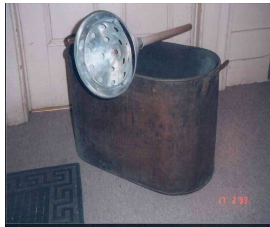
Showing the inside of the plunger which was used to agitate the clothes being washed in a tub when no washing machine was available.
